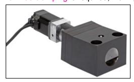
industry and in clean rooms. Because all functions are monitored electrically, the wedge clamps can be easily integrated into automated systems. The 24 Volt version of the wedge clamp offers high retention forces of up to 240kN with a current of just 3.8A. This makes the clamping elements particularly suited to systems in which dies and moulds have to be secured in tight spaces with high clamping forces.
