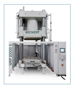
hook and placed into a rack for cooling. He then collects the new mould from the preheating station and pushes it into the machine on the roller strips. A lateral and middle centering device simplifies the positioning. Pressing the button again finally clamps the mould against the magnetic clamping plate.
