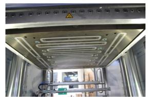
between 47 mm (without heating unit) and 85 mm with integrated heater, an option that Wickert prefers for all presses. The size and geometry of the plates can be freely adapted to meet the requirements of the application.
