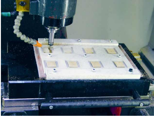
(GEL1.jpg and GEL2.jpg) Workpieces frozen securely on Triag triGEL worktable
