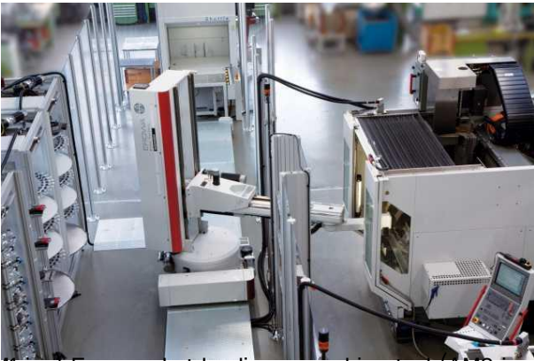
(AM1.jpg) Eropa robot loading a machine tool (AM2.jpg) Pallets of raw material ready for automated loading
