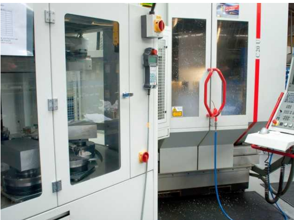
(AM3.jpg) Pallet system holding a variety of raw material ready to be automatically loaded and machined
