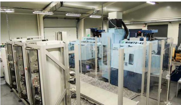
(AM4.jpg and AM5.jpg) Multi-machine tool cell supported by one linear robot
