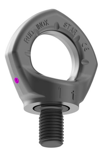
The INOX-STAR stainless steel eyebolt is made from a pentagonal shape and the body and the bolt is made out of duplex steel 1.4462; which offers a high resistance in sea water and across working environments with a high concentration of chloring ions. It also offers an impressive full working load limit in all load directions.
