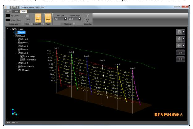
Renishaw's Cabled Boretrak and Rodded Boretrak borehole deviation measurement probes are designed to support a variety of drilling operations by providing vital borehole deviation analysis required to make fast and informed decisions. By using Boretrak to survey drill holes, any deviation from the intended path can be measured, monitored and addressed in order to achieve safer and more efficiently planned drilling and blasting.
