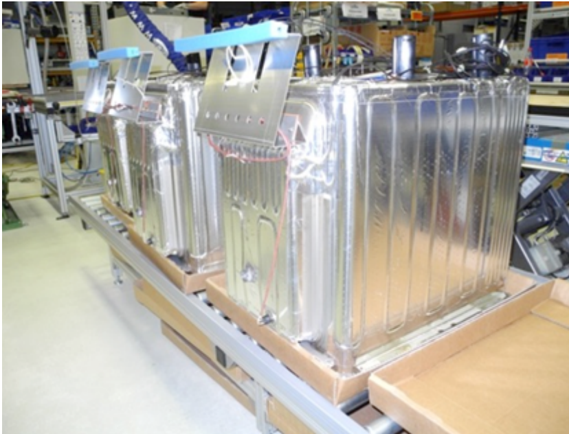
Photograph 7: When the heater foils are attached and the sensor and fixture are mounted, the inner containers wait to be insulated and enclosed in the outside casing.
