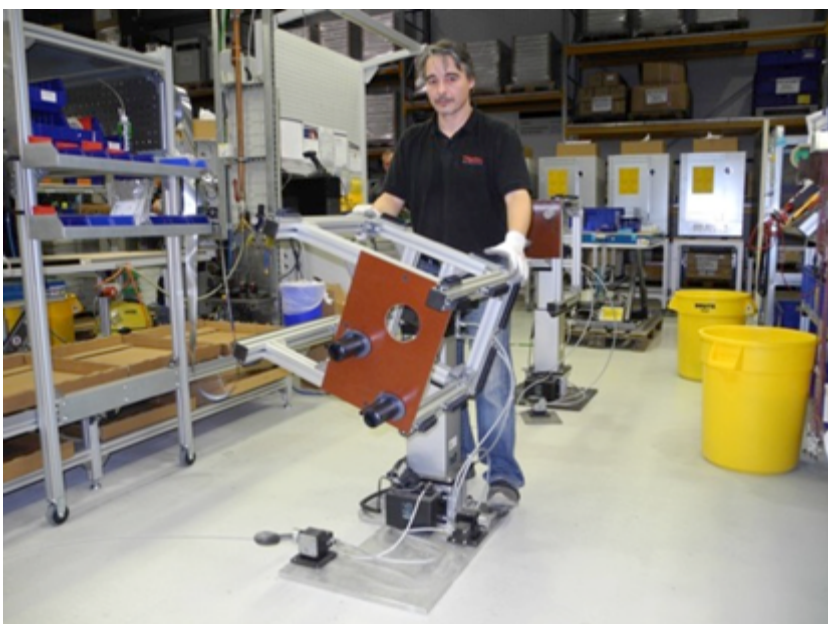
Photograph 1: All workstations have an electronic Shop-Floor lift module which is lifted and lowered by means of a pushbutton, and a rotary module operated by means of two foot switches.
