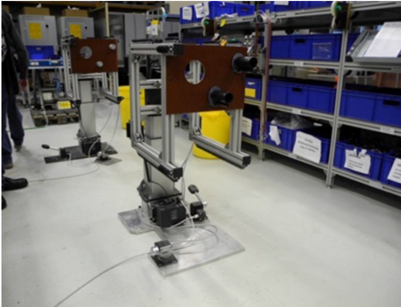
Photograph 1: All workstations have an electronic Shop-Floor lift module which is lifted and lowered by means of a pushbutton, and a rotary module operated by means of two foot switches.
