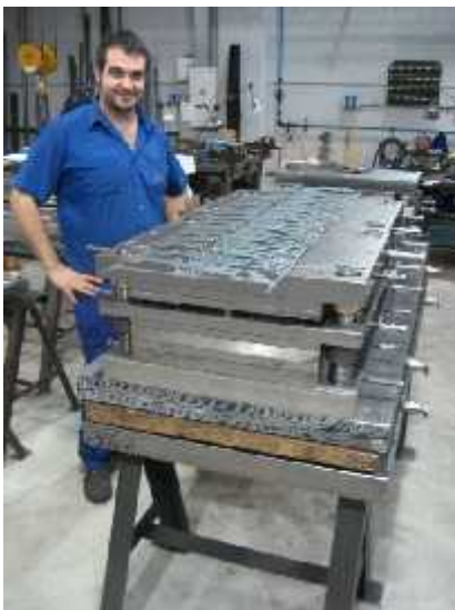
Fig. 3 Piece for electronic car system made in a Progressive die containing Toolox 44 parts
