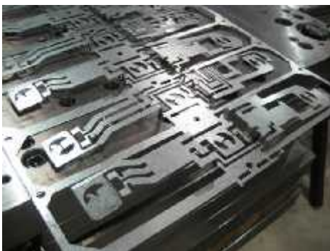
Fig. 3 Piece for electronic car system made in a Progressive die containing Toolox 44 parts
