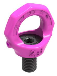
The STARPOINT VRS also known as the STAR among eye bolts offers many advantages. Firstly the STARPOINT will swivel to the direction of the load lift, the working load limit is therefore always at the
