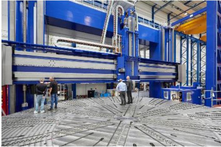
HACO's new gantry portal milling machine will allow for effective and efficient turning, milling and drilling of even very large components of high-strength welded and cast steel
