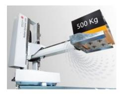
So now all EROWA system sizes can be exchanged from the individual magazines. Grab the exchangeable fork gripper and it ensures a secure lift up to 500 kg. and with the RCS5-gripper, the Robot Dynamic 500 can now load all other Erowa pallet sizes too.
