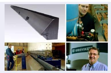
Ursviken Pullmax produced this 3 metre long pressbrake blade in Toolox 33 and measured only 0,7mm maximum deflection from end to end. Milling speed was also 25% faster than with the previous material 1.2312 (P20 with Sulphur).
