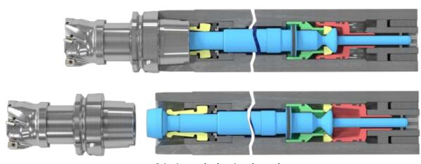
Gripping and releasing the tool
