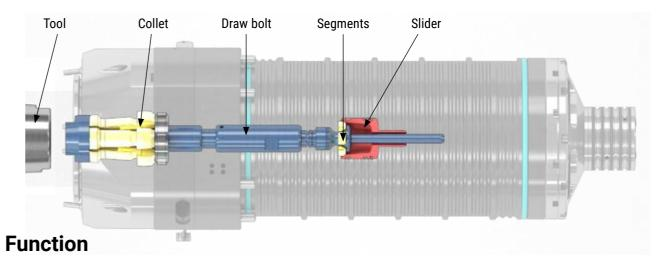
The clamping system for clamping the tool is actuated hydraulically. The tool is retracted and positively locked via clamping slides, locking segments, draw bolt and collets.
