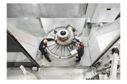
The Dörries VTL enables complete processing in one set-up of many typical pump components (housings)
