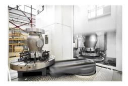
The Dörries Contumat VCE 2000 vertical turning lathe, with a pallet table and separate table and motor-driven alignment stand, allows the set-up process for the next workpiece to be completed while another is being processed
