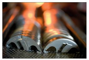
Sintering of powder compacted parts.
