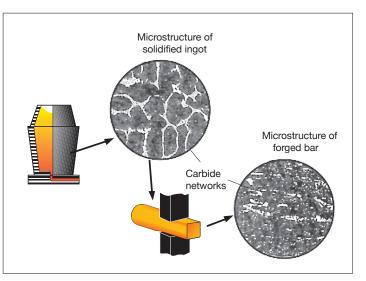
Figure 5. Breakdown of the carbide networks during hot forming.
