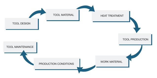
Figure 1. Factors influencing tool life in cold work applications.
