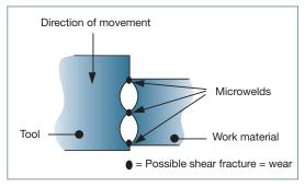
Figure 4. Schematic representation of adhesive wear.
