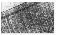
Photo 1. SEM photograph of a D2 punch worn by abrasive wear (work material 1% C-steel at 46 HRC).
