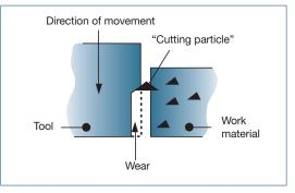
Figure 2. Schematic representation of abrasive wear.
