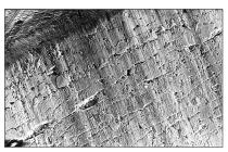
Photo 2. SEM photograph of a D2 punch worn by adhesive wear (work material austenitic stainless steel).
