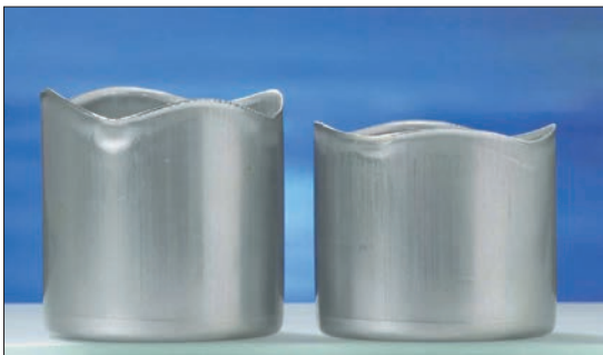
The influence of lubricant viscosity on drawing. Maximum cup height using lubricant viscosity 500 cSt (left cup) and 40 cSt (right cup).
