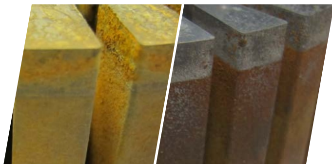
Die Cast Mould cleaned
