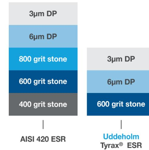
You are able to achieve a high-gloss surface (SPI A1) in three easy polishing steps, resulting in 40-50% less polishing time compared to standard tool steels such as AISI 420 ESR.
