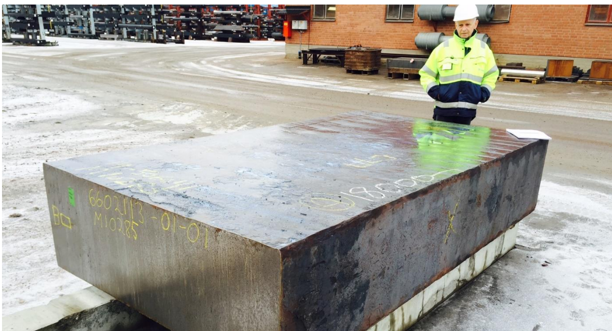
Figure 8 shows just how big some special sizes of Uddeholm Dievar can be manufactured
