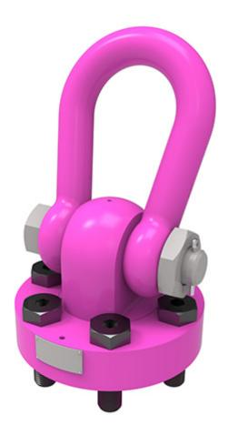
The WBPG is loadable from any side in the direction of the pivot meaning it is suitable for lifting and turning of heavy loads. It has the ability to rotate 360° and swivel 180°. The WBPG comes with a detachable suspension ring in the shape of a shackle for the attachment of common lifting means.
