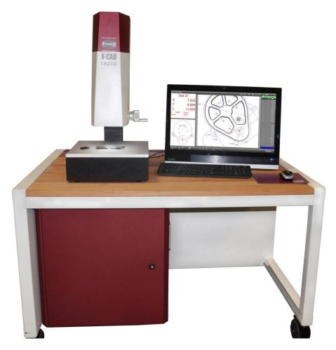
Spectrum Metrology is pleased to introduce the new workshop VideoCAD Rapid system, a high definition 2D measurement device which offers unsurpassed speed: the acquisition and analysis of measured data takes only a few milliseconds. Its unique combination of touch-screen software and fixture free workstage allows detailed measurements at the touch of a button. This approachable design means that 100% throughput inspection is now a reality.
