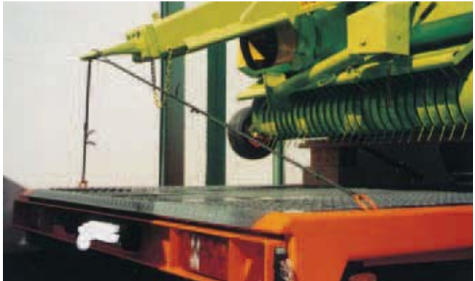
Twisted wires and worn out lashing means result in a big risk!
