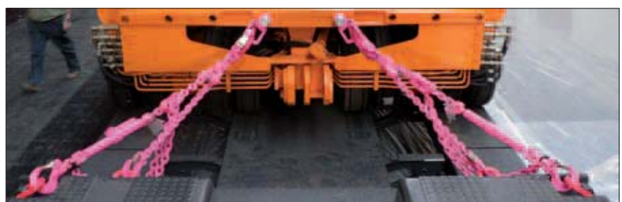
Four bearing strands by VIP lashing chains with special balancer rolls
