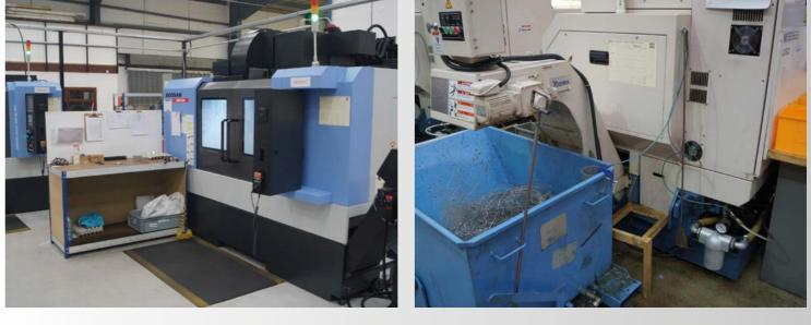
collects the cutting fluid which is normally dragged out of the machine tool by the swarf that is evacuated by the automatic chip conveyor or swarf auger and wasted. The neat oil or water miscible (soluble oil) cutting fluid is reclaimed by siphoning it from the chip-container and returning it to the machine tools main coolant tank for reuse.
