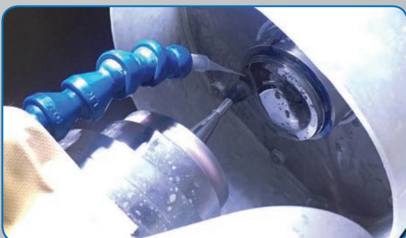
The Mould being Polished on an IRP 50
