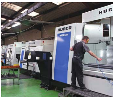
A Hurco VMX64t with an X-axis of over 1.6m: The most recent CNC machining centre to be installed at Crossen's Belfast factory
