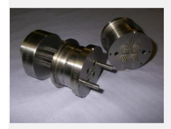
A four-impression mould tool from ND Precision designed for quick changeover in the production of electrical/electronic connectors, (Source: System 3R)
