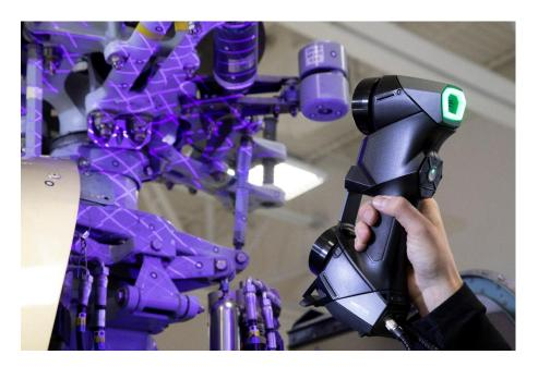
When complex or large environments need to be recorded, or small manufactured parts need to be inspected, laser scanning can provide a convenient and cost-effective solution to data collection.
