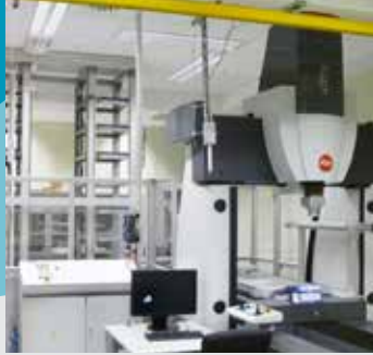
This parts buffer holds waiting parts and is configured to sit behind the Leitz PMM-C High Accuracy CMM.
