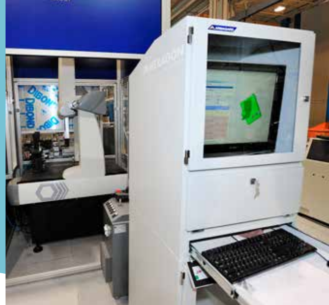
A CMM from Hexagon Metrology measures blades that were placed on a mount (left side of the granite table) by a robot outside the enclosure.
