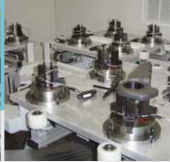
This parts buffer is composed of four pallets. One pallet at a time is loaded onto the CMM, located in the inspection room.
