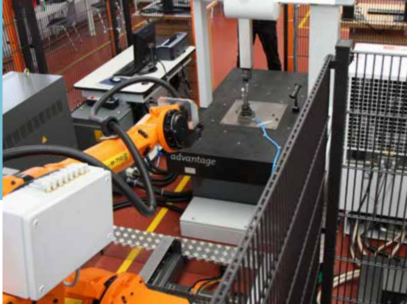
A GLOBAL CMM in an automated EDM cell is loaded and unloaded with a slide mounted robot.
