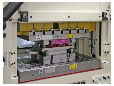
Because the entire clamping surface of the magnetic plate is metallic, no costly standardising of die sizes and clamping edge heights is required. Roemheld magnetic die clamping plates are suitable for vertical and horizontal use in machines and for all die sizes and shapes, even non-standardised ones.
