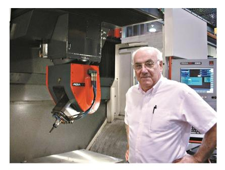
This cell comprised a modern machining centre for milling graphite electrodes and a WorkMaster robot from System 3R. The cell can hold 140 finished electrodes in a rotating magazine. A single operator handles all the preparations for the electrodemaking process - electrode design, programming and operations list. The operator knows which electrodes may be critical in a process and when the EDM machines need electrodes, so that machining can run smoothly as it has done for nearly 20 years!
