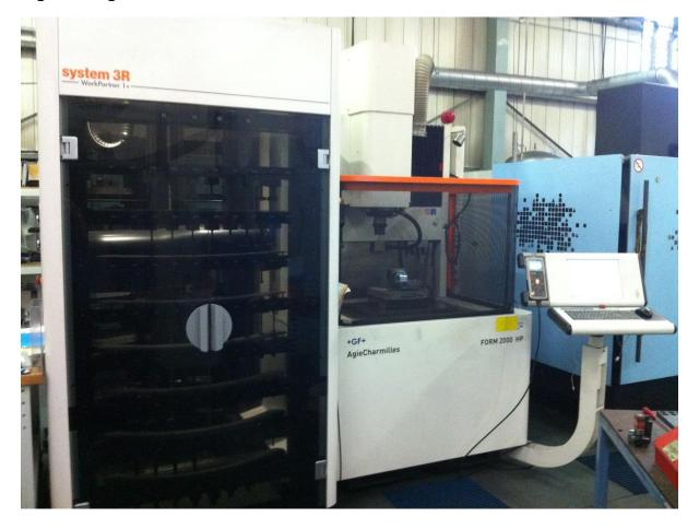
By investing in the very latest technology, they have automated their spark erosion cell by combining a System 3R WorkPartner robot with their
