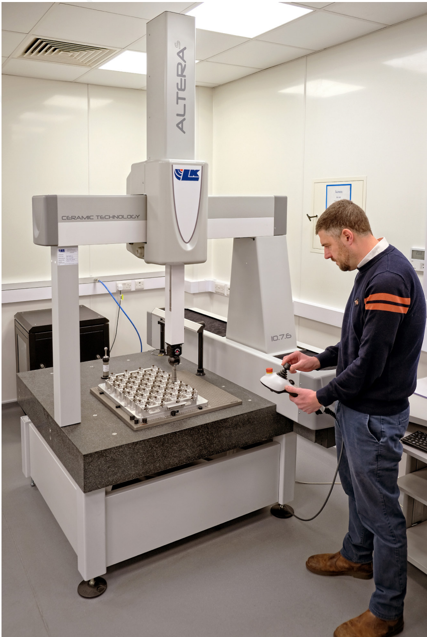
Peter Makosa setting up one of the reduced-height LK Altera S CMMs in the temperature controlled inspection room at Alltrista’s Christchurch factory in the UK.
