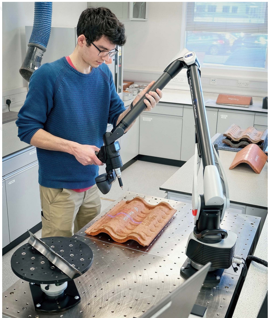
Another view of the tile being laser scanned, with the LK FREEDOM Index Table in the foreground
