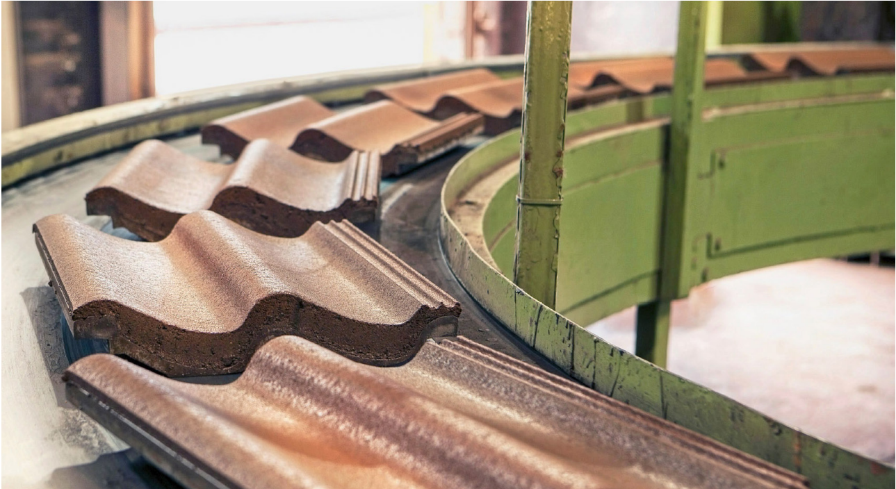
Concrete roof tiles on a production line at BMI Group's Shawell manufacturing facility in Lutterworth, UK.
