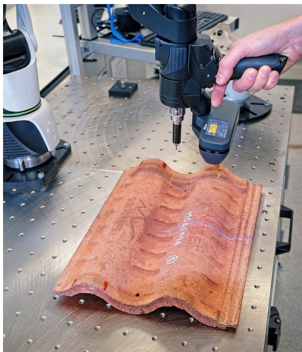
Close-up of a tile being laser scanned
