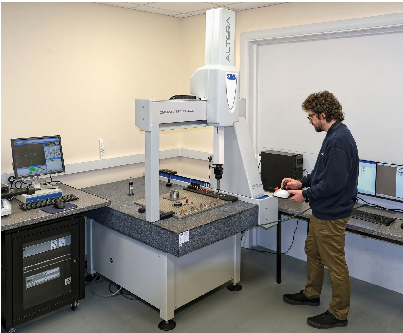
The British-built Altera 10.7.5 has a volumetric accuracy of 1.3+L/350 \mu\text{m} , where L is the measured length in millimetres
