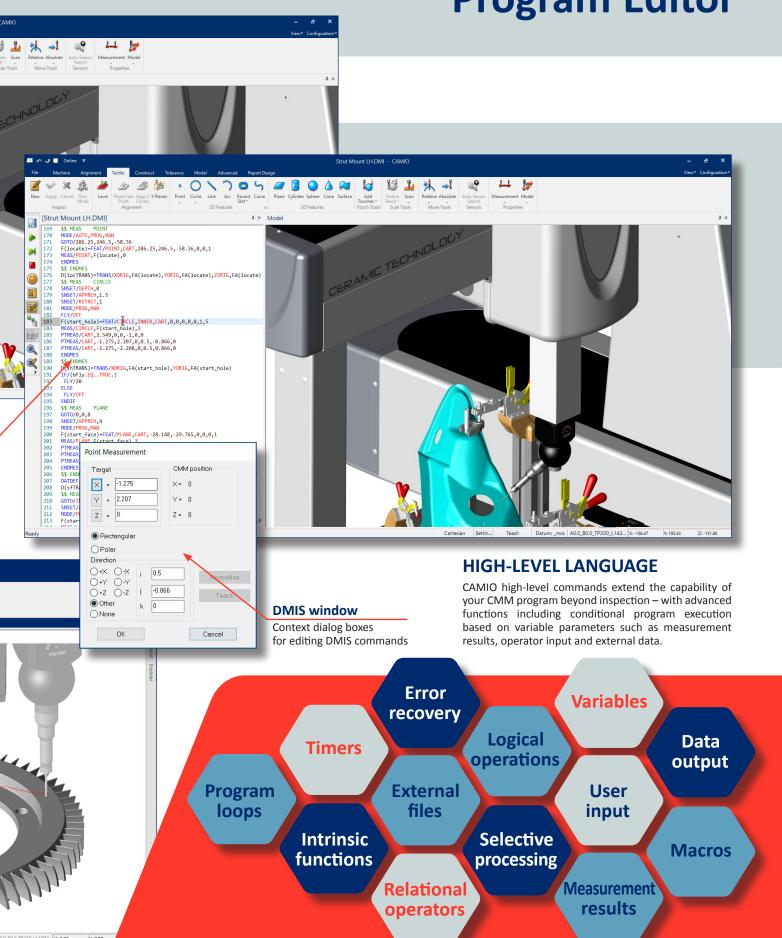
CAMIO simulation allows programmers to fully prepare programs and optimise measurement sequences offline – ensuring programs are ready before parts arrive for inspection, and dramatically reducing CMM downtime when proving out programs.
