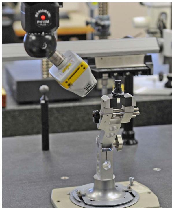
Laser scanning the plastic body of an ABS speed sensor using a digital laser scanner on an LK ALTERA CMM
