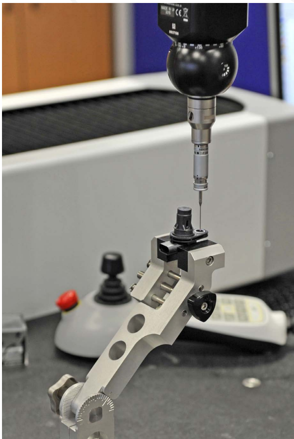
Tactile probing the ABS sensor body.
