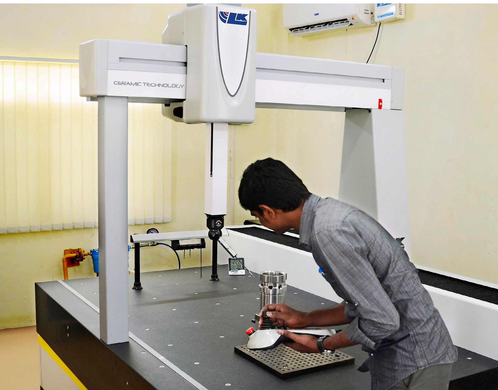
A Fine Forge CMM operator setting up inspection of a turbine blade on the LK Metrology ALTERA CMM using the continuous scanning probe.
