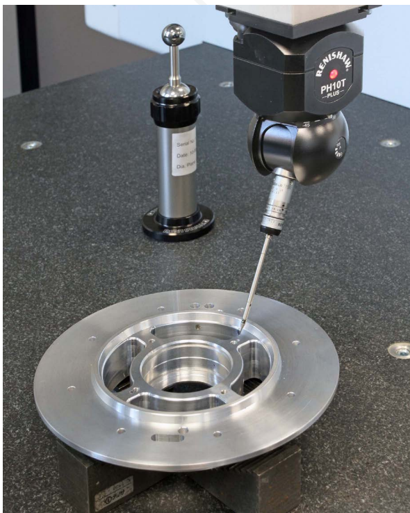
The aluminium turbine component being inspected in a cycle time of 10 minutes
