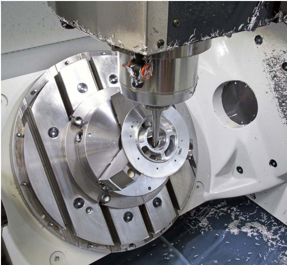
The turbine component being machined on the Spinner 5-axis vertical machining centre
