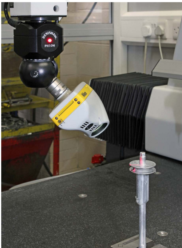
The laser head on the LK CMM scanning a zinc die cast actuator shaft for a Loadhog handling product
