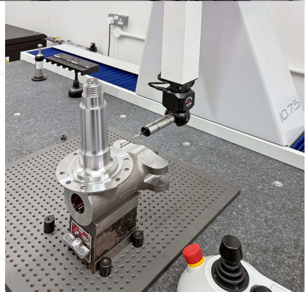
Two further images of the Spitfire axle being inspected
