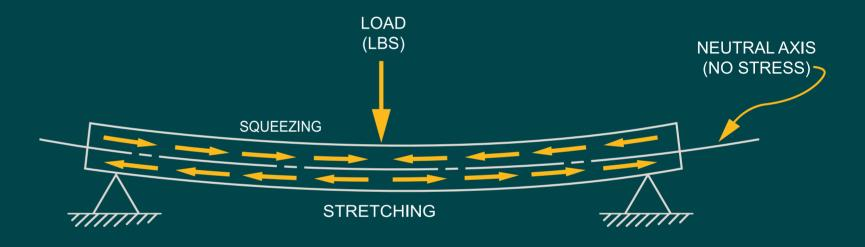
The flexural test measures the force required to bend a beam under three-point loading conditions - providing an indication of a material's stiffness when flexed. The data is often used to select materials for parts that will support loads without flexing.
